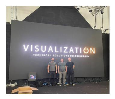
Direct-view LED technology has many advantages which meet the specific requirements of the church. The solution offers an extended half-life of 100,000 hours, compared to the previous projection system's 20,000-hour half-life. This increased longevity significantly reduces maintenance costs and ensures a longer-lasting investment for the church.
